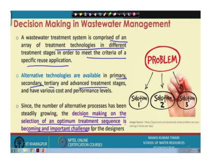
So, this is basically what is the concept of fit for purpose water uses and this for the purpose it is used. So, this brings us to the decision making, because we are at if we see. So, a wastewater treatment system is comprising array of technologies as we are saying that there for the fit for purpose water treatment, based on the output level will have to select a treatment train or will have to select a treatment scheme.
