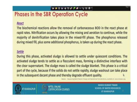
Then we go to the next stage which is react so react stage is the typical stage where these biochemical reactions takes place that is why we call it react. So, those bio chemical reactions which allow the removal of carbonaceous BOD; the major objective of the waste water treatment is the removal of the dissolved organic matter or soluble BOD that way. So, those organic matter which kind of produces this carbonaceous BOD are removed ok.
