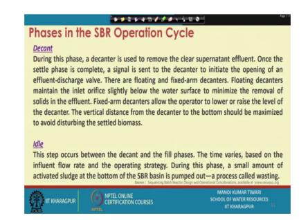
Now, the next cycle is the decant phase. So, during this decant phase a decant is typically used which is kind of set or given the objective of removing the clear supernatant effluent ok. So, the treated waste water is separated from the sludge mass in this decant stage. So, once this settle phase is complete, this is the next step after the second phase; once the settle phase is complete a kind of signal will be sent to the decanter to initiate the opening of the effluent discharge valves.
