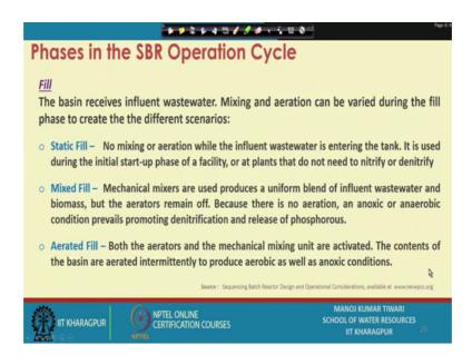
So, if we see these different cycles in the first cycle which is the filling ok. So, in the first cycle there is the fill is just the basin your batch basin will receive the in front waste water ok. So, again as you are saying mixing and aeration can be varied in this filling
