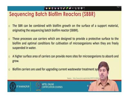
Now, up gradation of this SBR is the sequential batch biofilm reactors which are SBBR ok. So, these SBBR can be like sort of combined system where the SBR and biofilm growth takes place together. So, what happens in SBR we have a suspended growth system right the water is comes in a tank, and then we have make certain radiators. So, growth takes place in a suspended fashion there is no media. So, there is no possibility of biofilm growth ok.
