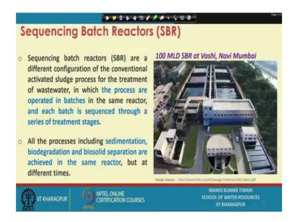
So this sequencing batch reactors or SBR, what typically we call are kind of a different configuration of the conventional activated sludge process. So, what happens in a conventional sludge process, we have the waste water coming in after a primary sedimentation or a primary settling tank. And thereafter it eventually goes to the next
