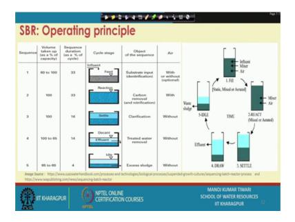
So, if we see the operating principle, o we have various sequences ok. And then that volume taken up as a percentage of the capacity, so the different volumes this sequence durations ok. And these are the cycles influent coming in this fill cycle, then reaction, then settle, then decant, and then idle cycle. The objective here is to (Refer Time: 24:40) input ok.
