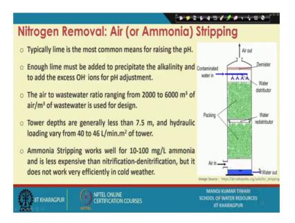
So, typically kind of lime is the most common means for raising the pH lime is added. So, that pH is raised. There is enough lime must be added to precipitate the alkalinity and to kind of increase the OH ion for the pH adjustment. The air to water ratio ranges from 2000 to 6000 meter cube of air per meter cube of wastewater which is typically used in the design and this works well for 100 to so, 10 to 100 milligram per liter range.
