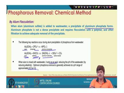
Whereas alum precipitation with the alum. So, where aluminum sulfate or what typically we call as alum is added to the wastewater and here a precipitate of this aluminum phosphate forms ok. So, these alum reacts with the this thing and a precipitate of this alum phosphate forms.
