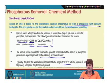
So, then there are couple of chemical approaches for phosphorus removal as well. So, the biological approach was the one that we discussed. Chemical approach it is actually a simple chemical precipitation. So, either lime based precipitation or alum based kind of
