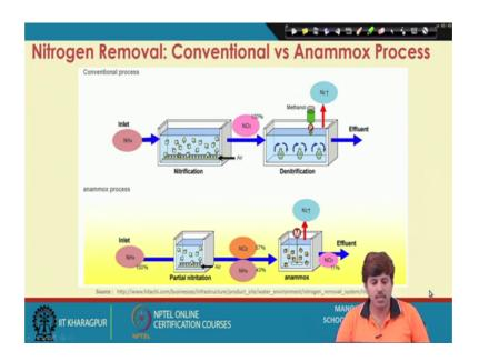
Now if we compare it with conventional processes when conventional processes we have ammonia coming through a nitrification basin and then converting into the nitrate which is going to the denitrification releasing night nitrogen and effluent. And in the process it needs a methanol or some organic carbon source.
