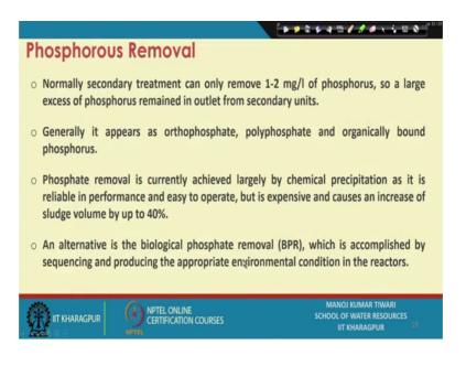
So, that kind of aerator is there. This is how typically stripping system looks like. Another nutrient that is there in the water is phosphorous which kind of normally secondary treatment can remove 1 to 2 milligram of phosphorous. So, a large excess of phosphorous still remains in the outlet of the secondary unit. The there is kind of different forms of phosphorous. It could be in the form of orthophosphates, polyphosphates or originally bound phosphorus.
