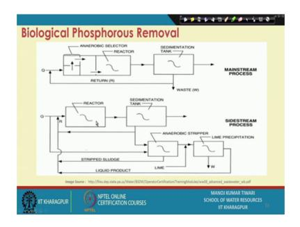
So, there are kind of it there are mainstream processes where we can have anoxic reactor followed by in kind of aerobic system right away or we can have a side stream process, where this anaerobic process done is in a side stream. And, then actually it is again supplied to the conventional aerobic system that way.
