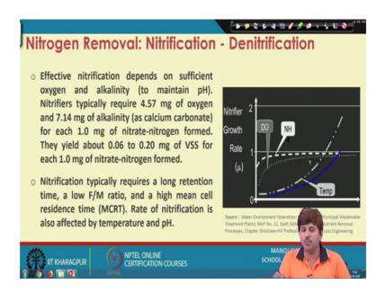
The effective nitrification depends on kind of sufficient oxygen and alkalinity that should be present in the system ok. So, typically this nitrifier requires 4.57 milligram of oxygen and 7.14 milligram of alkalinity as a calcium carbonate for each milligram of nitrate nitrogen formed. And they you usually yield from 0.06 to 0.2 milligram per liter of biomass or VSS for each one milligram of nitrate nitrogen which is being formed in the process of nitrification.
