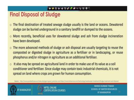
So, this brings us to the final disposal of sludge where the sludge is finally, disposed off. This final destination of the sewage sludge is usually the land, or the ocean the dewater sludge which we get can be buried underground in a sanitary landfills, or can be dumped to the ocean.
