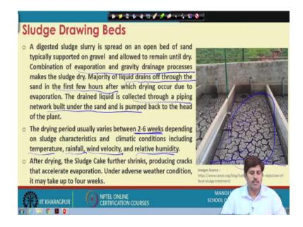
Then the sludge drying beds which are there, so it a typical sludge drying bed will traditionally look like this ok. So, this is kind of a sludge drying bed. Now what happens that the digested sludge slurry, slurry which comes after the sludge digestion and conditioning which is an optional step, but if you provide conditioning; so, the condition sludge is spread on a open bed of sand and typically a kind of supported on gravel and allowed to remain until it becomes dry ok.
