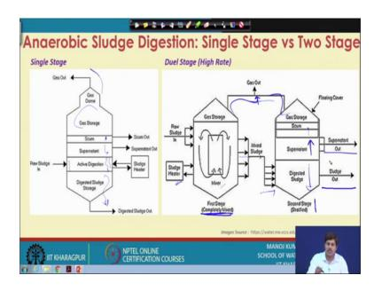
So, that will be basically a high rate digestion high rate digestion and low rate digestion. We have single stage and two stage or what we call as duel stage digestion as well. So, in a single stage digestion again it is typical process as we were just looking at. So, we will get raw sludging, there will be active digestion, there will be supernatant, there will be scum formation, then gas storage, and gas can be taken digested sludge will come at the bottom.
