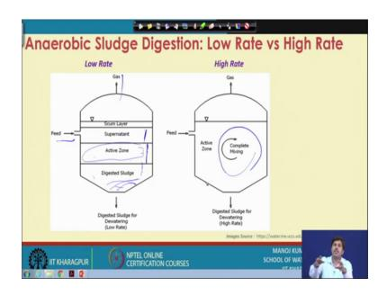
So, as we said that this digestion could be low rate, or high rate digestion process. So, what happens in a low rate digestion? If we see the feed that we get in the feed that we get in eventually comes to a closed chamber because it is anaerobic digestion. So, there will be like there will be active zone where this sludge gets digested and that once it gets digested it will try to settle it will come to the lower zone.
