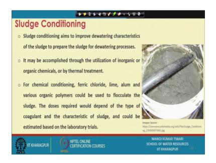
So, a post stabilization what we see is the sludge conditioning ok. The sludge conditioning aims to improve the dewatering characteristic. So, what happens? If you recall the process that we saw in the earlier class, so sludge is first thickened and then it is stabilized.
