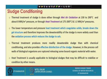
Then we have thermal conditioning of this sludge this thermal conditioning of sludge is done either in wet air oxidation, or what we typically call as through heat treatment. So, there are two approaches out of which heat treatment is far more popular as opposed to the wet air oxidation.
