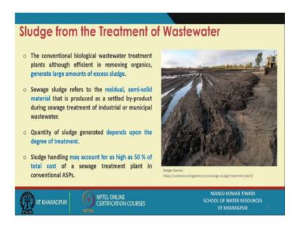
So, that way we end up generating sludge from the various different units in the treatment plant. Now what essentially is sludge? The, it is the conventional wastewater treatment plant although quite efficient in removing the organic matters, but at the same
