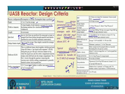
Now, if we see the various design criteria ok, so the design criteria again there is reactor configuration, it can be rectangular or circular. If we see the physical parameters over here, so it can be rectangular or circular ok. Rectangular shape is generally preferred. The depth is 4.5 to 5 meter for sewage treatment. The width to diameter is the inlet length of the literals are around 10 to 12 meter.
