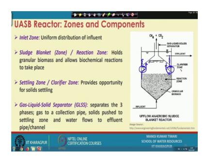
Of course, there are some other components like there would be a what we call is deflector. So, this kind of deflectors would also be there ok, which deflects the flow and does not allow the flow to basically directly pass through the openings across the gas-
