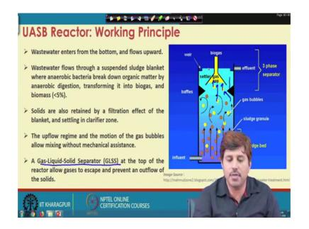
So, as we are discussing the role of GLSS is to separate or to phase out the gas liquid and solids from the reactor from the material or mass which is coming up. So, what happens that this deflector helps the gas bubble not to go directly, but to basically it deflects the gas bubbles and solid particle along with the water to this zone. And then the gas will once it is deflected, it will rise up ok. So, this gas bubbles that way go up, and then there is a gas cap or gas trap.
