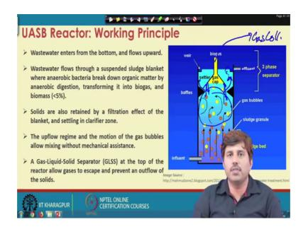
And through this pipe or tube, this gas is collected. So, this goes to gas collection system eventually. So, our gas is separated, it is got collected or it is got basically separated away from the water. Now, what happens to the solid and liquid over here, water here, so solid particles also basically rising up.
