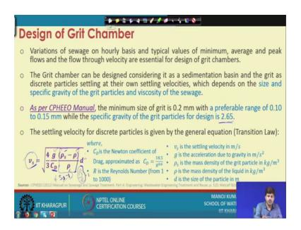
Now, if you go for the design of grit chamber, the design of grit chamber is primarily based on the settling of the particle, because as we discussed, it is the prime objective of a grit chamber or grit removal system is to let the heavier grit particles settle in the chamber. So, variations of the sewage on hourly basis and typical value of minimum, average and peak flows are first estimated ok, and then the velocity essential for the design of grit chamber is calculated based on that.
