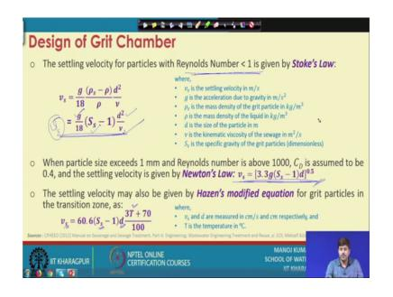
Now, for the design practices, because we do not know the C D in the we just were seeing that slide earlier here. So, since C D is not known to us ok, we are we do not know what is actually the value of C D over here So, without C D, we cannot estimate the settling velocity. So, we start from an approximation, and to begin with, we consider the settling velocity of the particle with Reynold number less than 1, which is typically given by the Stoke's law.
