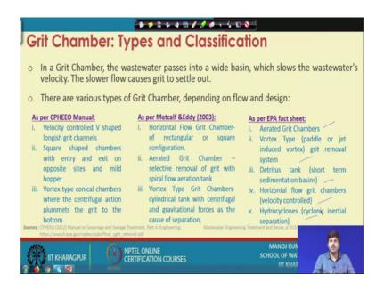
EPA fact sheet proposes few more types of grit chamber. So, there is aerated grit chamber, there is vertex type, which could be paddle or jet induced vortex. There could be detritus tank, which is short term sedimentation basin kind of thing. Horizontal flow grit chamber, which is based on the velocity control and there could be hydro cyclones, which is cyclonic inertial separation of the grit from the water. So, there is various principles, which work on such systems for the removal of grit.
