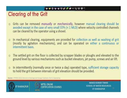
Now, how we clean grit. Typically, can be removed manually or mechanically; however, manual cleaning manual clearing of the grit should be avoided in case of a large STPs. If your STP is very small say less than 1 MLD, so the amount of grit deposited is not that high. And one can go for manual cleaning, but in the larger STPs or larger treatment
