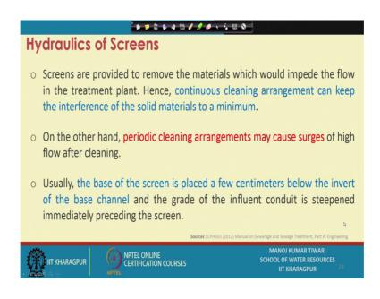
Then, when a water channel is passing through the screen there is going to be certain had hydraulic disturbances. So, his screens are provided to remove the material which would impede the flow of the treatment plant, ok. So, if we are in a flowing channel, if you are putting obstruction in the form of screen, it is obviously, going to the disturb the flow conditions, ok.
