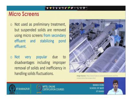
So, these are not in fact, a screen that we have been discussing so far. As a first unit, they can be used at a later scale and they are not very popular due to several disadvantages that improper removal of solid and inefficiency of holding solid fluctuations. Because, with if the solid load comes more, these screens probably will not be able to withstand that load and that is why, it is not that popular.
