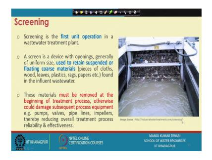
So, screening is the first unit operation in a water treatment plant. We are saying it unit operation because, it is a purely physical process, ok. There is no chemical reaction or nothing is involved in this, ok. So, screen is typically a device with opening generally of the uniform size which is used to retain this suspended and floating course materials.
