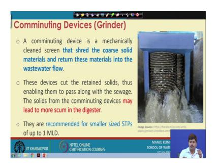
Commuting devices or grinder is actually again a mechanically cleaned screens. What it does? It shreds the coarse solid materials. So, you are seeing here these kind of setups
