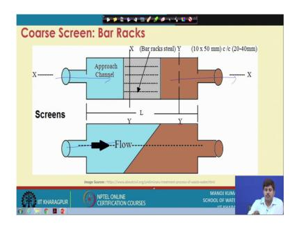
So, if we see the screenings process, so, let us say this is our approach channel, ok. The water is flowing in like this and then we have the different bar racks here kept at the stake and then the flow is in short that way. So, since it is kept typically kept on inclined and particularly the manually clean one so, if you see the front view, it will look like that where wastewater is flowing like this and if you see the top site, it will look something like that.
