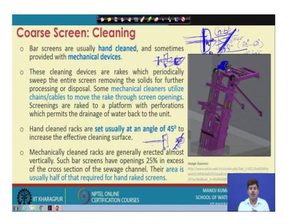
Now, the cleaning process of screens are of like very essential because it is efficiency will depend on the cleaning. Otherwise, if you do not clean and things get accumulated on the surface of screens. It could get choked and it will it may actually prevent the flow itself, ok.
