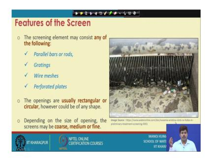
Now, if you see the features of a screen. So, the screen elements generally consist of either parallel bar or rods, it could be greetings, it could be wire mesh, it could be perforated plate. So, those kind of things can be used for the screening purpose. It is just simple physical filtration, ok. The openings of these screenings are usually rectangular or circular. However, technically it could be of any shape. It could be of hexagonal, pentagonal so, that way, like it could be of any shape.
