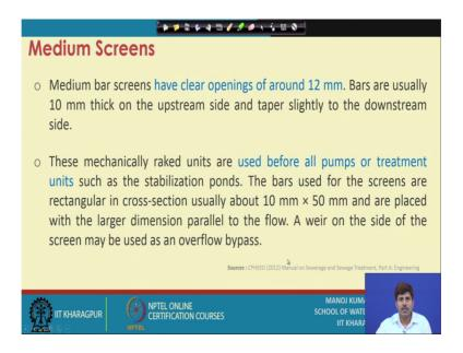
Then, we have medium screens medium bar screens have clear opening of around 12 mm very less use though these are typically 10 mm thicks on the upstream side and tapper slightly towards the downstream side. These are mechanically racked units mostly and used before all pumps or treatment unit so, as to things can get protected and should not allow to pass in through, ok.
