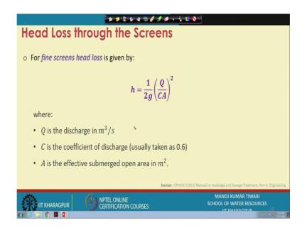
There is for fine screens, we use typically this formula for head loss estimation, 1 by 2 g cube by C A square. Here, Q is the discharge in meter cube per second, C is the coefficient of discharge which is usually taken as 0.6 and A is the effective area of the opening in meter square. So, this way, we can estimate the head loss through the screens, ok.
