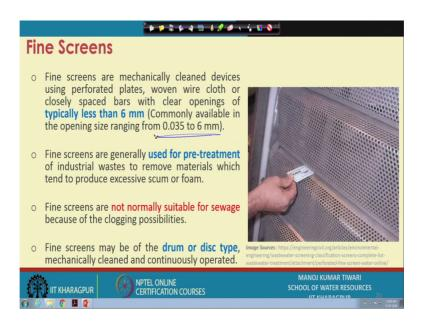
And, then the fine screens which are again mechanically clean devices. Because it is not possible to practically clean such devices manually. Depending on the size, they are typically less than 6 mm opening, but commonly available opening range is from 0.35 to 6 mm, ok. So, 35 micrometer to 6000 micrometers are the actually range of the opening, the fine screens are generally used for pretreatment of industrial waste to remove the materials which can forms come or form.
