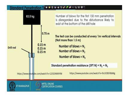
So, first one I have discussed about the; standard penetration test. So, that where a borehole is required in the borehole we are placing a speed spoon sampler tube and with the drill rod we are applying hammer blows on the speed spoon sampler tubes and we penetrate that sampler tube into the soil and then we count the number of blows required for 150 millimeter penetration.
