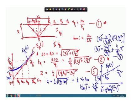
So, this is the wave that is the source and here we have one geophone or that is the receiver and we have another soil layer. So, this is the layer I this is the layer II and as I mentioned we can generate the P wave or S wave depending upon how we are applying the hammer blows.
