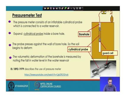
So, and then the next one we discussed about the pressure meter test where, cylindrical probe is inserted into the borehole and the pressure is applied with the application of the pressure, the volume of the probe, or the cavity or the borehole increases. So, that volume increases measured;
