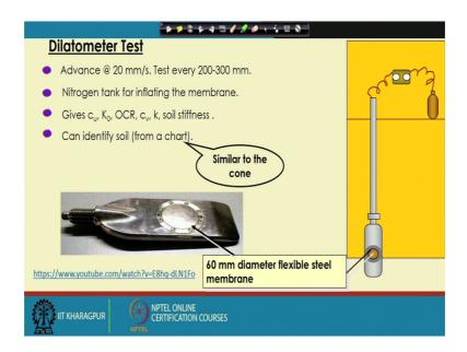
Similarly, we next we discussed about the dilatometer test where the nitrogen tank is used; so to inflating the membranes. So, here where which is similar like a pressure meter test, where this is the flexible membrane which where the inflating which is this membrane is inflating with the help of the nitrogen so, that resistance the pressure initial pressure and the pressure after the expansion is recorded.
