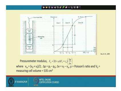
So ultimately we will get pressure versus a volume curve and from it this curve we identify 2, 3 different zones and from 3 different zones, we got p 0, p f value and p l value. So, with the help of this p 0, p a value and v 0 and v a value ah; we got the
