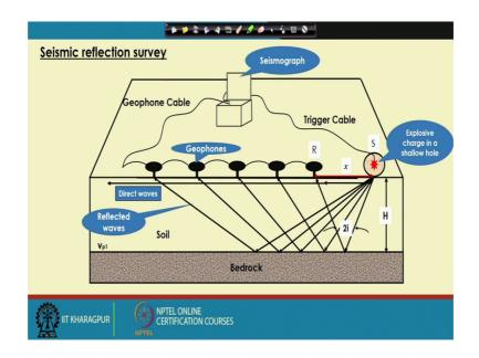
Because the procedure of this seismic first I am talking about the seismic reflection survey. So, the procedure is that we there is a source where we are generating some wave and we are placing some receivers which are called geophones at different intervals. And from this source the wave which is generated will be received by this receiver. So, these receivers we are also placing on the surface and the source is also on the surface.
