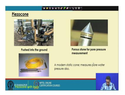
Next one is a Piezocone. So, nowadays the with the static cone we measure the pore water pressure also because here the pore water porous stone, for the pore water pressure measurement unit is attached. So, we can measure the cone resistance, we can measure friction resistance, we can measure pore water pressure and we can re measure the friction ratio.
