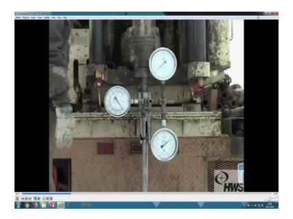
So, these are the testing methodology, here we are measuring the resistance that this is the estimate and this is it is pushed into the soil. So, once we get the resistance, then the next step we have to determine the soil properties, we those properties will be required for our foundation design.
