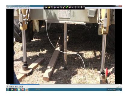
So, it is pushed and then the corresponding readings are and then we increase the depth of the or increase the depth of the instrument by attaching the this rod and then we can measure the data.
