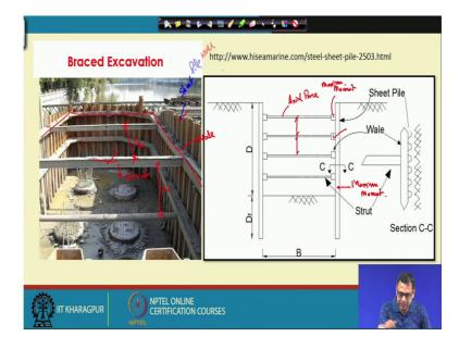
So, what is the brace excavation? So, brace excavation is that as you have observe the sometimes these the depth of the sheet pile will increase if your height of the sheet pile is more.
