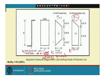
So, this is the p a value of the p a or it is equal to 0.65 gamma H into K A or where K A is equal to 1 minus sin phi divided 1 plus sin phi or this is tan square 45 degree minus phi by 2.
