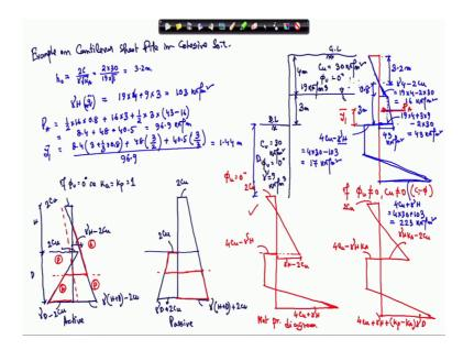
I have solve one example problem on cantilever sheet pile in granular soil and anchor sheet pile in granular soil. Now, this class first I will solve one example problem on cantilever sheet pile in cohesive soil ok. So, I am taking the similar kind of example problem that I have solved during the granular soil. So, this is the dredge level, this is dredge level and this one is the ground level ok.
