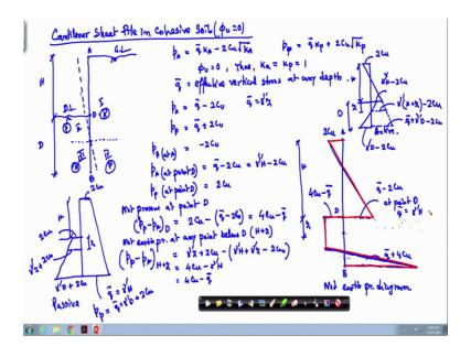
That is phi u is equal to 0. So, in the Cantilever Sheet Pile in Cohesive Soil; again it is assume that this is the gl, and this is the dredge level that your point of rotation will be any point below the dredge level and above the base of the wall.
