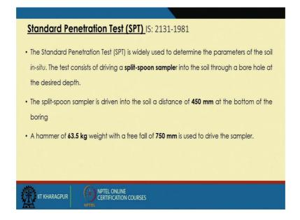
So, what is the standard penetration test. So, as I mentioned it is an indirect method. So, the standard penetration test is widely used to determine the parameters of the soil or in situ soil, the test consists of a split-spoon sampler into the soil through a borehole, at the desired depth.
