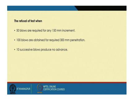
So, next one is that that when the refusal of test. So, now, if the fifty blows are required for any 150 millimeter increment or 100 blows are obtained for required 300 millimeter penetration or 10 successive blows produced no advance, if any of them occurs then we will stop this test because you cannot proceed further with this test.
