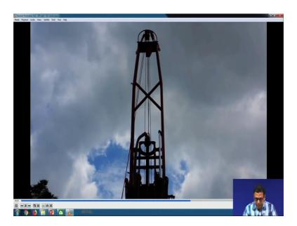
We apply the hammer blow, and then we count the number of blows required for each 150 millimeter penetration and this is the sampler tube. So, it is collected now.
