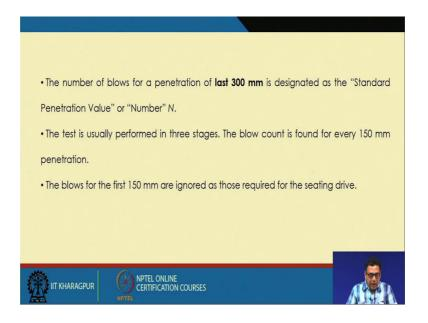
So, the number of blows for a penetration for last 300 millimeter is designated as the standard penetration value or the number N.
