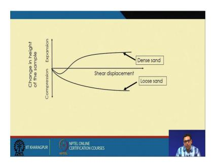
So, what will happen that in the dense sand, your volume first decreases then increases and loose sand your volume continuously decreases; So, in case of dense and your volume increases. So, dilatancy means that increase is in volume due to the shearing or the.
