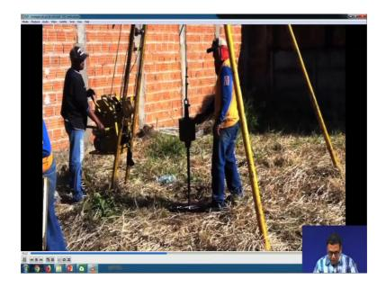
So, hammer weight is 63.5 kg, free fall is 75 millimeter, here this is the drill rod and where these hammer blow is applied and in the bottom of this drill rod, this sample of tube is attached. So, this is the another way we can conduct these SPT test.
