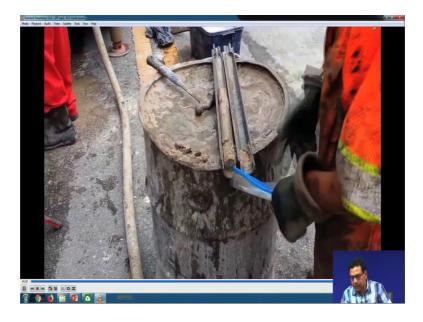
So, the advantage is that in this test, we are collecting the soil sample as well as we are measuring the N value or the SPT value. So, this soil sample which we are collective, we can use it to determine the soil properties to the laboratory test as well as we can we have the N value, that N value we can use to determine the soil properties also.
