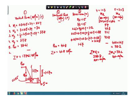
And so, I will make a table with the first I will make a vertical forces. The unit is kilo Newton per meter, then the horizontal forces unit is again kilo Newton per meter then I will take lever arm lever arm is meter. Then I will take MR that is a resisting moment kilo Newton meter per meter and MO over turning moment kilo Newton meter per meter.
