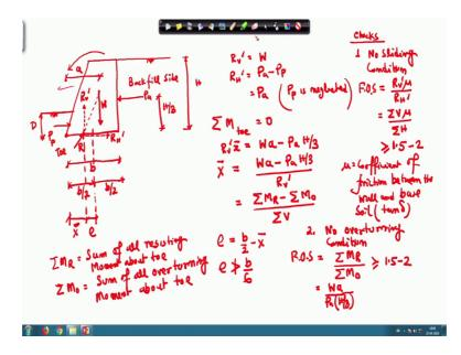
So, these are the things that as was I was discussed then this is the factor of safety and then no sliding condition, this is the factor of safety and no overturning condition.
