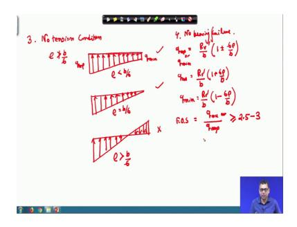
So, next one the third one is the no tension condition. So, there should not be any tension developed in the base of a retaining wall as I mentioned that you can see that there is eccentricity. So, that means, the stress distribution below the base of the foundation of retaining wall is not uniform, because the as there is a eccentricity. So, forces or stresses may be more will be more in one side and will be less in the other side.
