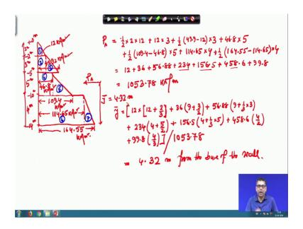
So, I will first separately I will quickly I will I am drawing that diagram again, and then I will calculate the force. So, this is minus 2 meter, this is minus 5 meter, and this is minus 10 meter, and this is minus 14 meter. So, this is the diagram cause this is 12 then there is increase, then there is a decrease of the diagram, then again increase it is increasing then again increasing and finally, this was the diagram ok.
