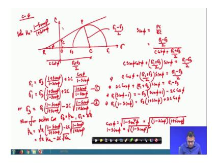
So, now if it is a c phi soil then I can write or I can draw this Mohr circle, but here it will not pass to the origin because it has a c value as well as the phi value. So, this is the phi value and this one is the c value cohesion. And this is the, your Mohr circle and this is again this is sigma 1, this is sigma 3, this is the center.
