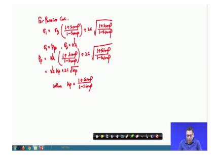
So, I have expression sigma 1 is equal to sigma 3 1 plus sin phi 1 minus sin phi plus 2c root over 1 plus sin phi 1 minus sin phi. And for the passive case your sigma 1 is equal to P A and sigma 3 is equal to gamma z. So, I can write sorry this is P P. So, I can write that P P is equal to gamma z 1 plus sin phi 1 minus sin phi plus 2c root over 1 plus sin phi 1 minus sin phi . And again gamma z into K P plus 2c root over K P where, K P is equal to 1 plus sin phi 1 minus sin phi 0k.
