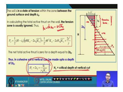
So, I can write that P A is equal to gamma z K A minus 2c root K A equal rights small a or capital A. So; that means, here if your up to the z 0 this is negative part is more compared to the positive part. After that it will into positive part will increase. So, up to this point there will be a negative earth pressure; that means, here attention will. So, this is the negative means if the tension. So, this is the tension zone so, ok.
