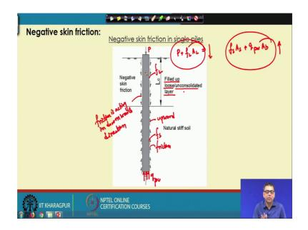
Now, what is negative skin friction ok? So, when we talk about pile load shearing mechanism where, if we apply the load on a pile the resistance will be given to the pile by keep resistance or bearing and then the friction. So, this is the tip resistance of the bearing and this is the friction.
