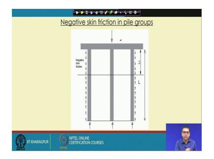
So, this is the previous calculation is for the single pile, now if it is the group pile in the clay the same way we can calculate. So, this is the group pile configuration.
