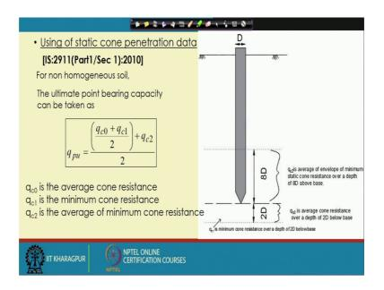
That I have discussed about the this cone static cone penetration data using this static cone penetration data to calculate the pile tip resistance and the frictional resistance. In that day I solve one problem with a particular cone resistance data along the depth.
