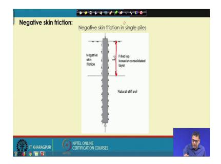
So, this is L c and then this is the perimeter of the pile and they see that mean this is the area of the top portion of the pile, where the negative skin friction is developed into alpha into c u. And, similarly for the cohesion less soil also we can calculate the similar way. This is the center portion of the top uncompressible layer, we have to calculate the lateral stress so, and into tan delta.
