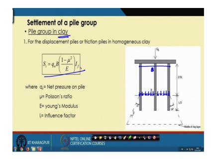
So, next one the settlement calculation of pile group it is also very important. So, till we are talking about the load carrying capacity of the pile group. Now, this is a settle how we will calculate the settlement of a pile group.
