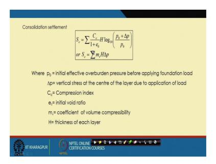
This is for the consolidation settlement and these terms are same exactly that we used for or sallow foundation calculation. But, remember that the raft you have to place at two third from the top of the pile cap. And then influence zone will be twice of the width of the pile from that two third of the a length.
