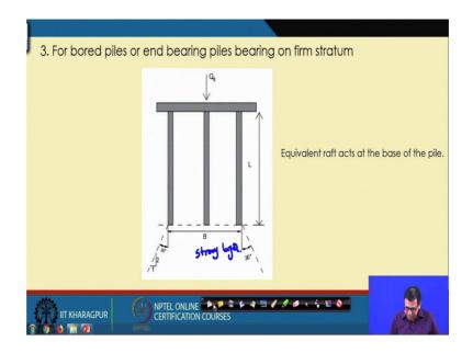
And then if this pile is rested on a very strong layer because, this is the very strong layer. The soil is very strong and pile is rested on the strong layer. Then form that base you have to place the you have to distribute the load and at that base you have to place the raft.
