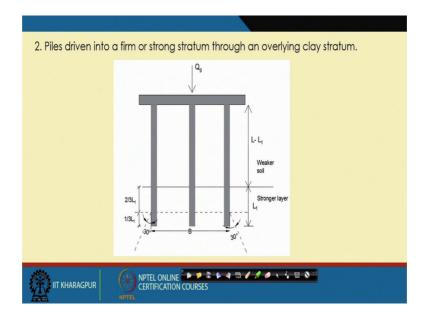
And then if suppose this upper layer is very weak soil lower layer is very strong soil. But, previous one is the homogeneous clay but, here the upper layer is very soft but, the lower layer is very strong ok.
