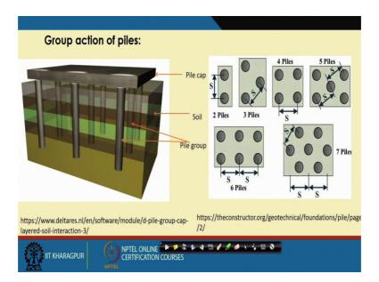
Is the group action of pile, the till now I have discussed the pile load carrying capacity based on a single pile. But, pile will be used as a group.
