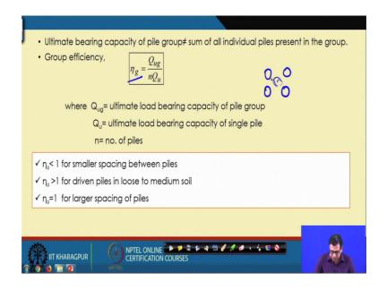
So, now the how we will calculate the efficiency of a pile group that the efficiency of a pile group is the group load carrying capacity of pile divided by number of piles into the single load carrying capacity of pile.
