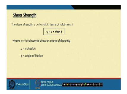
So, first we should know that, what is shear strength of a soil. So, the shear strength of a soil is can be represented by cohesion plus sigma n tan phi. So, this is the is a sigma n, this is sigma n which is the applied normal stress on the soil.
