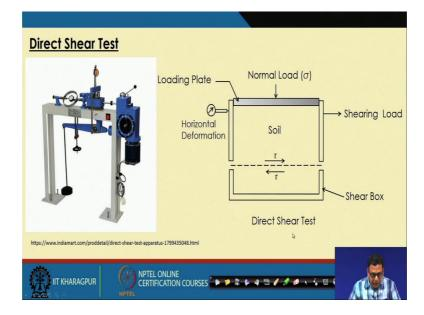
So, now so, this is the first test this is the direct shear test. So, in the direct shear test we have a direct shear test box, where it has two halves. So, it is basically a horizontal load is applied. So, we apply a shearing on in the soil sample.
