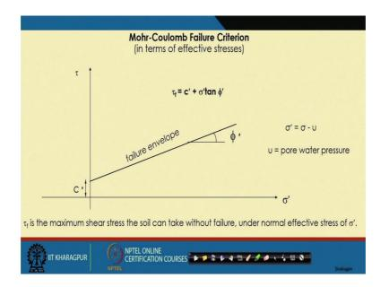
We can write thus similar type of expression, which is c prime plus sigma dash, tan phi dash. Here these is sigma dash or sometimes it is written as sigma bar is the total stress minus pore water pressure.
