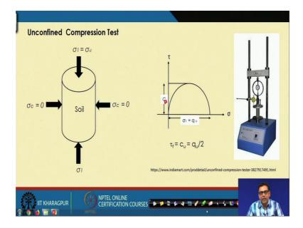
The next one that we are talking about is the unconfined compressive compression test. The major difference between the unconfined compression test and the triaxial test, that in the triaxial test we are applying a sigma 3 or sigma c that mean the all down pressure around the soil through the water. But here sigma 3 or sigma c value is 0, we are not applying if you look at this sample here we are not applying any stress around the soil we are not applying any pressure.
