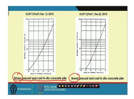
So, this chart first chart is for the driven piles, driven precast and cast in situ concrete piles if the pile is driven pile. Basically driven piles and driven piles in both can be the cast in situ and the precast. So, for the driven pile we use this chart and for the bored pile we use this charts. So, again here we are separately we can calculate the driven pile and the bored pile.
