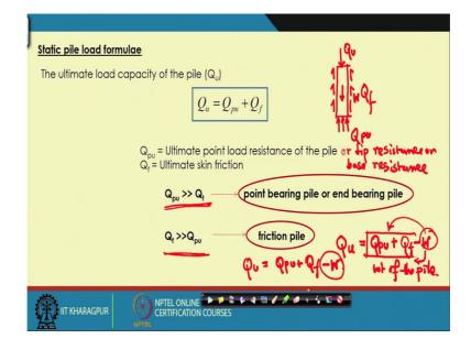
So, first I will use that static pile load formulae so, that ultimate load carrying capacity of the pile can be defined as Q is the ultimate load carrying capacity Qpu plus Q f. Where Qpu is the ultimate point load resistance or sometimes it is called tip resistance or it is called base resistance. So, that means, as I mentioned that when you are applying a load on a piles. So, you will get the resistance from this base or the tip, or you will get the resistance from the friction, ok.
