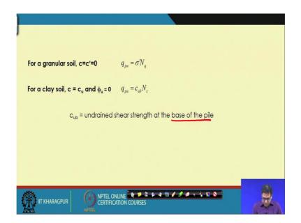
Now, for granular soil if c is equal to 0, then qpu will be sigma n Nq sigma prime Nq, and for the clay soil this qpu will be c u at the base and Nc. So, it is at the base, remember that. So, this will be the at the base of the pile, and then the Nc.
