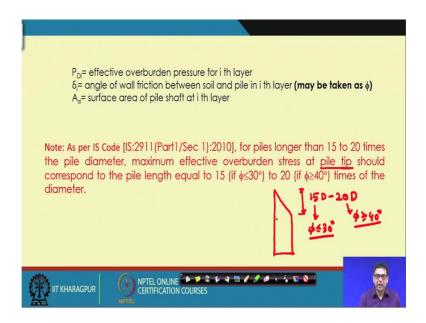
And the, this is the and delta is the fictional angle here it is IS code has recommended, that it can be taken as a equal to phi, ok. And other things are are so, this is that your this is the diameter of the pile this is a bearing capacity factor Nq n gamma.
