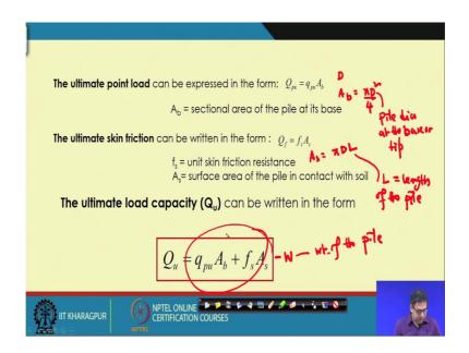
So, the ultimate load resistance is I will calculate in this way that Qpu small qpu, p u into Ab, A b is the base area of the pile and friction; that means, the friction resistance and the total area of the outer surface of the pile. And that is the so, that is mean here if the diameter of the pile is D, then the Ab will be pi D square by 4 ; where D is the pile diameter at the base or tip, ok. And here As will be pi D L, ok, where L is the length of the pi, ok.
