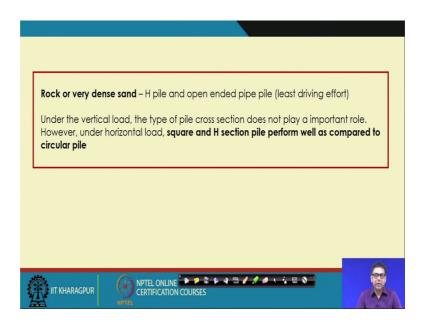
And so, for the rock and heavy dense sand H pile and open ended pipe pile is suitable and the all this example I am giving this is the suitable this is not the only application this is the suitable, but you can use the other kind of pile kinds of piles also, but this is one of the example where it is more suitable.
