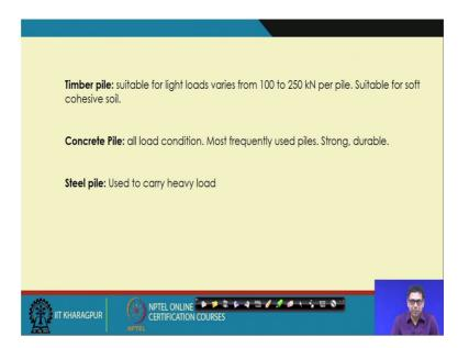
Now, when we will use the timber pile? So, it is suitable for light loads when the loading is very less or comparatively less varies from 100 to 250 kilo Newton per pile and suitable for soft cohesive soil because then it is very easy to drive into the soil was if the soil is very hard, then the pile may be this timber piles maybe damaged because of this because your soil is very stiff you are applying the driving force. So, it will there is a possibility this piles can be damaged.
