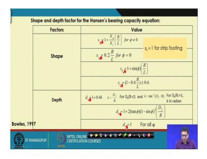
So, one way is that if the H B is parallel to the width axis, then the way that I have discuss you have to determine in that way. So, that will be the all factors suffix B and if the horizontal load is parallel to the length axis even if H B is 0, then you calculate the factors in two ways one is considering the B, another one is you replace the B with L and the L with B ok. So, that I have discussed so; that means you will get two factors.
