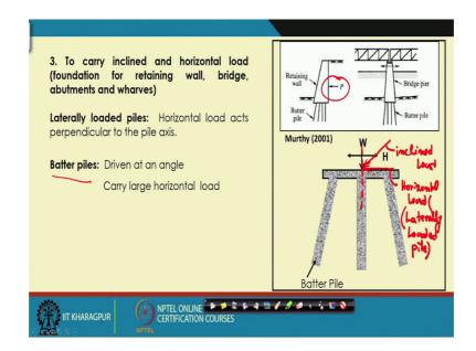
Say then the in the next type of pile based on the loading is called the pile can be subjected to inclined or horizontal load. So, that type of if the pile is constructed below a retaining wall or bridge abutment or in the offshore where the waves are coming waves or the sea waves are coming which is in the form of lateral load. So, in those cases pile is subjected to horizontal or it can be subject to inclined load also.
