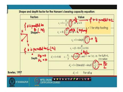
So, in case of Hansen theories that if the load is parallel to length direction so; that means, if we have the inclined load, now this inclined load has two components; one and one is vertical, another is the horizontal.
