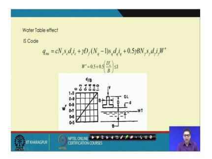
And, but if it is the IS method, then in the IS method it is recommended that if the water table is at the base of the footing then and above then it is always 0.5. So, the second term you no need to apply any corrections because it is mentioned that if it is above base of the footing, then it is always 0.5 and this is the W dash ok.
