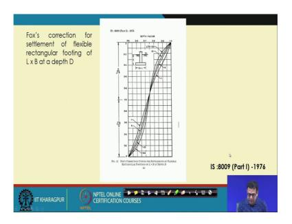
And this is the chart that I will use. So, this is a fox chart so, from here I will get the depth correction. So, the depth correction as it is mentioned you can see that D by root LB. So, this is D by root LB so, that is 0.67 so, 67 will be somewhere here so,
