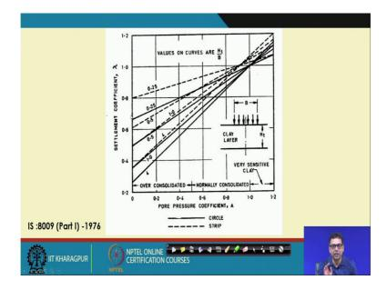
So, it is 2 so now, if I go to the chart then this is the chart where this is the correction factor. And here we are for the circular footing I am using because it is a square footing because here strip for circular is given. So, for that for normally consolidated soil this is
