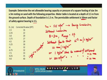
So, this so this is the problem; that was given the determine the net allowable bearing capacity or pressure of the square footing of size 3 meter cross 3 meter resting on sand with the following properties and water table location was 2.5 meter from the ground surface, depth of foundation was 1.5 meter, permissible settlement was 50 millimeter and the factor of safety against bearing was 2.5 and this is the N values were given.
