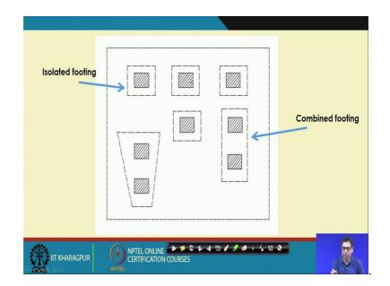
So, the next problem that I will discuss that foundation isolated footing on a on a on a clay. So, these are typical columns of a total building. So, what is isolated footing, if I if I if I design a foundation for a individual footing. So, there is a possibility that two footings may overlap.
