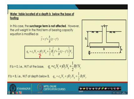
Now, keep in mind that if the water table is above the base of the foundation and at the ground surface then both the gamma will be gamma bar, if it is above the ground surface
