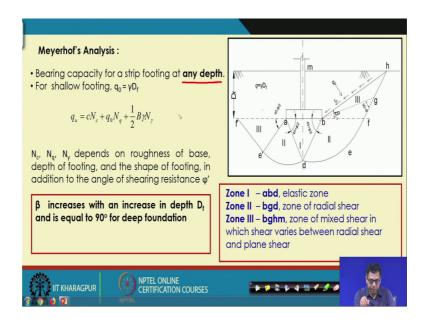
So, next analysis is proposed by the Meyerhof's where the this is also another advantage that each analysis we can use for any depth and this is further so, we can use for the this analysis and another advantage is that because in case of Meyerhof's analysis the N c N q n gamma that depends on the roughness of the footing, depth of the footing and the shape of the footing and the inclination of the loading in addition to the angle of shearing resistance phi.
