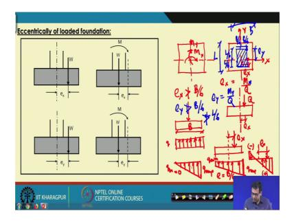
Next one that we are talking about that eccentrically loaded foundation. So; that means, we have discussed about the inclined loading. So, now, but if the in loading is inclined still the point of application of the load is at the center, but if the loading is not at the center it is some away from the center then how we will incorporated that thing into the bearing capacity expression.
