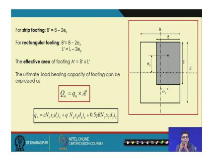
So, now this is the for the strip footing B dash is your, this is the area which is basically effective now because your footing is not in the center. If it is centered then your B is equal to B and L is equal to L because the total area is effective you are using the total area, but if your it is loaded in one side then your effective area that will reduce. So, this is the effective area because you are load is in the acting here.
