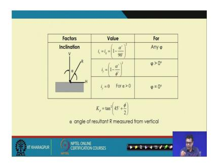
Here this alpha value is the angle the load is making this is the direction of the loading this R is the direction of the loading and it which alpha value and this loading making with the vertical angle. So, this is the alpha. So, this is and similarly K p value is given tan square 45 degree plus phi by 2.
