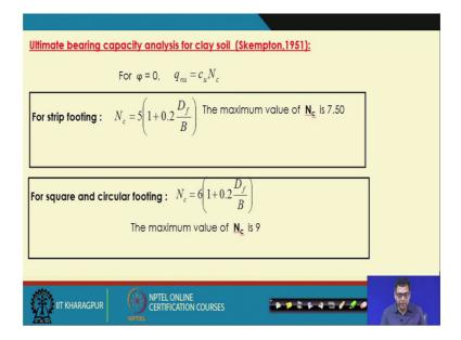
So, keeping in mind the Skempton 1951, proposed ultimate bearing capacity equation or theory for only clay, clay soils so; that means, here phi value is 0 and we are getting the net ultimate. So, that is the net ultimate. So, if the phi value is equal to 0 so, N q will be 1
