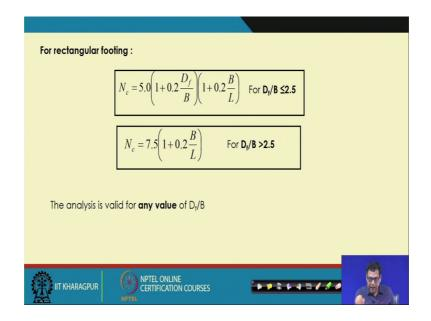
For the rectangular footing, we have this two equation; so, 1 D f by B less than equal to 2.5, then we have these equation and if the less D f by B is greater than 2.5 then we have these equations so, these equations where we can get the bearing capacity factor N c and that we can use for the equation which is given by the Skempton so, but this analysis valid for any value of D f by B.
