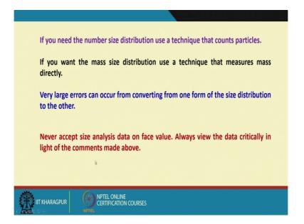
If you need the number size distribution use a technique that counts particles, if we want the mass size distribution use a technique that measure mass directly. Very large errors can occur from converting from one form of the size distribution to the other. Finally, I would say that never accept size analysis data on face value, always view the data critically in light of the comments made above.
