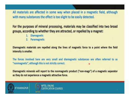
Actually all materials are affected in some way when placed in a magnetic field. Although with many substances the effect is too slight to be easily detected; that means, when any material you put it under a magnetic field, they have got some effect on this magnetic effect, but in some of the cases the effects are very pronounced in some of the cases, they affect our slide to be easily detected.
