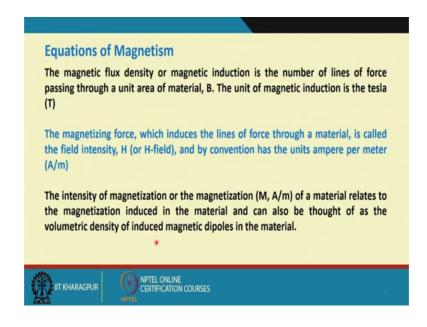
Now, just to recollect the basic physics regarding the magnetism applied to magnetic force. So, when it is applied to minerals, it is just a brief discussion on that that is called the magnetic flux density or magnetic induction is the number of lines of force passing through a unit area of material B.
