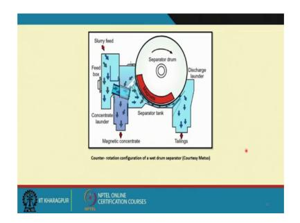
This is another design again by metso, this is based on your counter rotation that is slutty is fate through this and now the drum is rotated in this direction not in this direction and magnets are basically held up there. So, magnets are there. So, now, what will happen? Now when the it is moving in this direction so; that means, the material is being fade here and the magnetic particles are transported up to there and they in the as dislaws.
