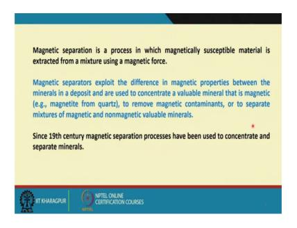
This magnetic separation is a process, in which magnetically susceptible material is extracted from a mixture using a magnetic force. That means, if I have a mixture of particles and if there are magnetic and non magnetic particles; that means, the particles which are susceptible to magnetic force and the particles, which are not susceptible to the magnetic force they are separated using a magnetic field.
