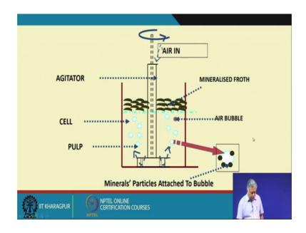
This is another demonstration how the particles get adhered to the bubble surface? So, you have got the agitator this is the same, this is the pulp, and now you have got this your air bubble and this is the, your demonstration the minerals particles get attached to the bubbles, and this is the mineralized froth and you have passed the air through this. This is again I have taken it from the open domain; I forgot to acknowledge this your source because I do not remember it right now.
