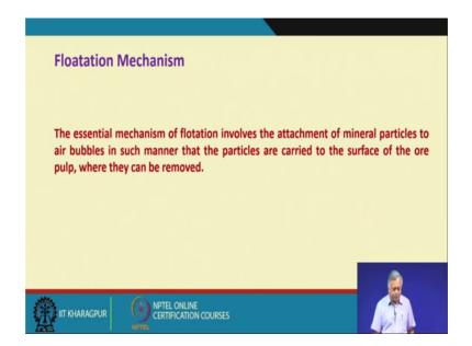
So, if you look at the essential mechanism of floatation involves the attachment of mineral particles to air bubbles, in such a manner that the particles are carried to the surface of the ore pulp, where they can be removed that is in the froth phase.
