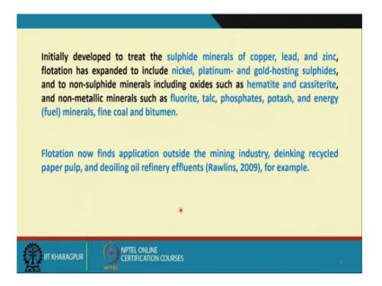
So, it was initially developed to treat the sulphide minerals of copper lead and zinc this was primarily developed targeting the processing of mainly copper and then also lead and zinc.
