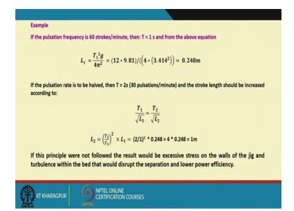
So, in the pulsation frequency is 60 strokes per minute. So, then t is equal to one second because it is 60 divided by 60. So, your what about the t? T is the period of pulsation. So, your t is equal to capital T is equal to one second and from the above equation.
