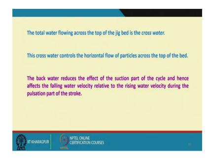
The total water flowing across the top of the jig bed is the cross water. That is when you are basically adding therefore, a because this normally the water moves in this direction. So, it have a vertical direction, but when you are arriving in this direction the water.
