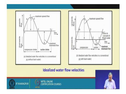
So, this is the compression stroke, that is your when you are compressing the in a in a Baum jig in a conventional jig, that is your when you are compressing it. So, the fluid is having a upward velocity and that is the maximum velocity zone. So, you are having a sinusoidal motion like this. So, this is the pulsation and this is the suction stroke.
