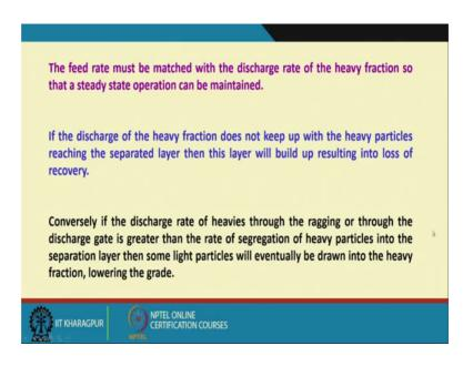
This is true for any continuous operation. If the discharge of the heavy fraction does not keep up with the heavy particles reaching the separated layer, then this layer will build up resulting into loss of recovery that is at what rate you are trying to remove the heavier fraction that is your wanted material.
