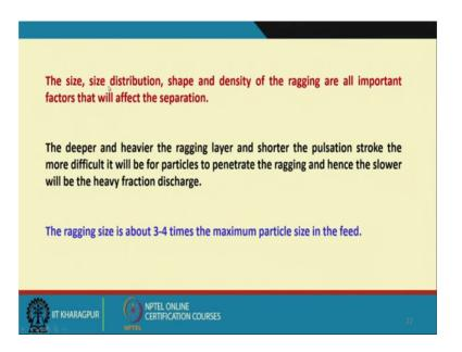
The size, size distribution, shape and density of the ragging are all important factors that will affect the separation. Even for the jigs where we are use ragging material. So, as the size of those particles size distribution because if you have wide size distribution. So, even the ragging material themselves, which are relatively finer they will occupy the wide spaces in between them.
