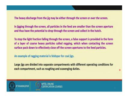
Now, the heavy distress from the jig may be either through the screen or over the screen that is what I have already explained you in the second slide. In jigging through the screen all particles in the feed are smaller than the screen aperture, and thus I have the potential to drop through the screen and collect in the hutch.
