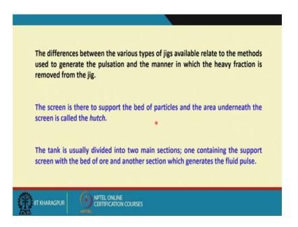
So, this is the difference between your earlier designed jigs and the presented jigs. The differences between the various types of jigs available relate to the methods used to generate the pulsation. Pulsation means the upward velocity and the manner in which the heavy fraction is removed from the jig; that is in case of coal the manner in which the clean coal fraction that is your float material is removed from the jig. So, what are the
