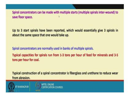
Now, what is the material of construction of spirals? Now spiral concentrators can be made with multiple starts that multiple spirals inter wound to save floor space sorry we will come back to the material of construction later on. So, that is like that that is you can have multiple stars like as I had shown you in the previous picture; that is you can have a stack of your spirals.
