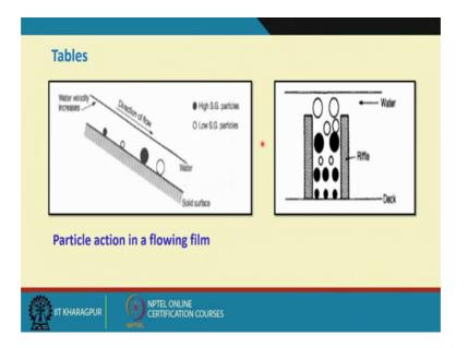
So, this is the tables in a particle action in a flowing film that is your I have already discussed about it that how it will work, but this is only explanation almost for some a few particles it is not that simple. When you are dealing with millions of particles it becomes little bit complicated, but that much of information is enough to understand whatever I have explained that how it works.
