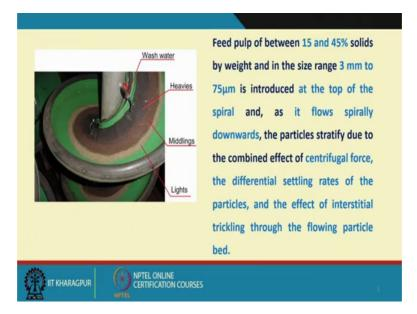
That, what is happening that you are we are feeding the material that is in the form of slurry and up from the top and then you have got a helical conduit like this.
