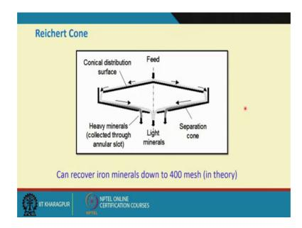
There is another version of this that is relatively modern design; improved design I would say of these flowing film concentrator; this word this is known as Reichert cone. So, here what we try to do we try to increase the capacity because you have seen that there the unit capacity may be less and what you try to do? You try to do it in stages like
