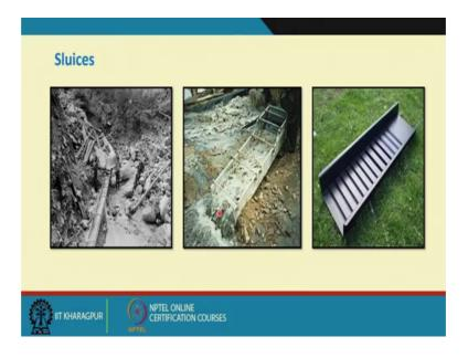
So, this was the earlier designs of the sluices, this is relatively your improved design what it is being tried that is suppose gold; gold when you have a free gold and so, they are in ppm level that is ppm level means it may be around 2 ppm or 3 ppm and if they are fine free gold so; that means, a 1 ton of material that is in 1000 kg of material, you are having on an average of 2 to 3 grams of gold.
