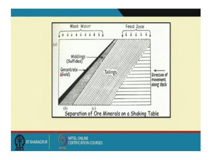
This is basically in detail of the how that table works and what is the wash water and feed zone direction of movement that is I said your deck also moves like this.
