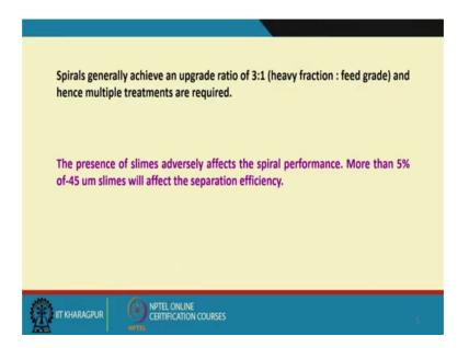
Spirals generally achieve an upgrade ratio of 3 is to 1 that is heavy fraction is a feed grade that is your ratio of up gradation is 3 is to 1 and hence multiple treatments are required; that means, in one go in a set of spiral that is you can have a upgrading ratio of 3 like it is analogous to again; that is what is your reduction ratio that is the instead of in place of crusher.
