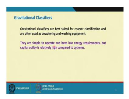
So, gravitational classifiers are based suited for a relatively coarser classification and are often used as dewatering and washing equipment.
