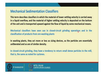
Then there are certain varieties of mechanical sedimentation classifiers, these term describes classifiers in which the material of a lower settling velocity is carried away in a liquid overflow, that is what I was saying that if I have lower settling velocity this will be carried in the overflow and the material of higher settling velocity is deposited on the bottom.
