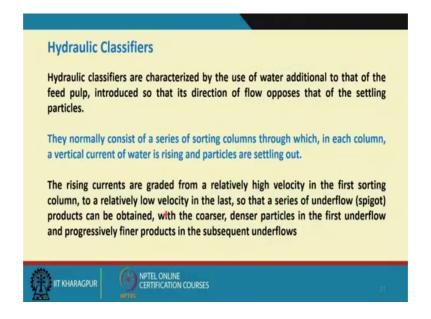
Now, there are another group of classifiers it is called hydraulic classifiers, the hydraulic classifiers are characterized by the use of water additional to that of the feed ball, introduced so that it is direction of flow opposes that of the settling particles.
