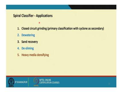
So, they have application in closed circuit grinding that is in primary classification with cyclone as secondary that is you can have a centrifugal separator after that. So, you are taking out you are removing majority of the coarser particles and then you have got relatively finer particles and you want have again a separation then you put it into a centrifugal separator.
