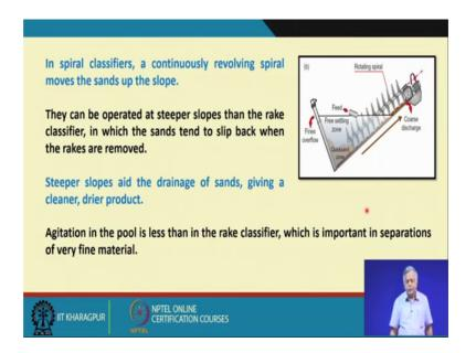
There is another variety of that is called the spiral classifier. So, in spiral classifiers instead of rake we are using a spiral. So, spiral actually is trying to transport your settled relatively coarser material which is settled; now when you are having spirals this gradient you can increase much than the rakes that is the mechanical aspect of that.
