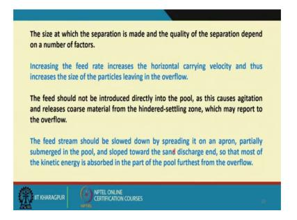
The size at which the separation is made and the quality of the separation depend on a number of factors what are those factors. Firstly, if we increase the feed rate it increases the horizontal carrying velocity because, you are feeding it at a very high rate because you are feeding the slurry.
