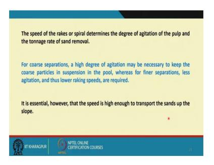
The speed of the rakes or spiral determines the degree of agitation of the pulp and the tonnage rate of sand removal. Now I want to make a quotient flow or I do not want to disturb the pool area, that is your I do not want to agitate the fluid in the fluid medium into the pool, for that I may have to run my rakes or you have spirals at a very slow speed, but the slow speed means your coarse are material removal rate will be less.
