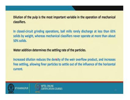
Is the most important variable in the operation of mechanical classifiers; that means, what is that maximum solid percentage in the feed I can have, that is very most important operating variable; in closed circuit grinding operations ball mills rarely discharged at less than 65 percent solids by weight; that means, what are the discharge we have we have got minimum 65 percent solids whereas, mechanical classifiers they were operate at more than about 50 percent solids that is by weight.
