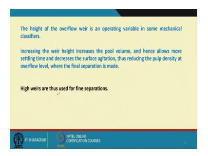
The height of the overflow where is an operating variable in some mechanical classifiers, the high definitely that is at what size of the if I need more finer particle to be at separation at much finer sizes, I have to increase the height because otherwise and if I can accept a little bit of course at your overflow then I can reduce the height. So, more height means lesser capacity and smaller height means more capacity, but at the expense of your quality.
