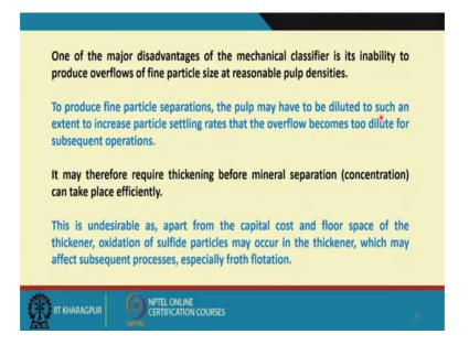
So, one of the major disadvantages of the mechanical classifier is it is inability to produce overflows of fine particle size at reasonable pulp densities, that is at a consistent pulp density; to produce fine particle separations the pulp may have to be diluted to such an extent to increase particle settling rates that the overflow becomes too dilute for subsequent operations, it may therefore require thickening before mineral separation.
