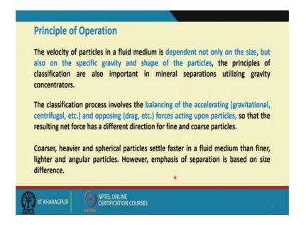
Principle of operation if you look at that is what I have already explained you. And if you go by these sentences that is what is written here there is the velocity of a particle; velocity of particles in a fluid medium is dependent not only on the size, but also on the specific gravity and shape of the particles. That is what we have discussed extensively during the lecture series on movement of solids in fluids.
