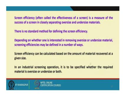
So, screen efficiency often called the effectiveness of a screen is a measure of the success of a screen in closely separating oversized and undersized materials. That is how effectively it has separated the oversized materials available in your feed and undersized materials available in the feed.
