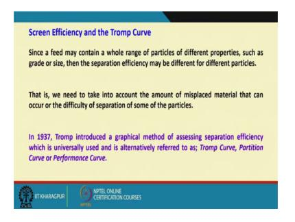
There are also other ways of looking at the screen efficiency. So, it is called the screen efficiency and the tromp curve because a feed may contain a whole range of particles of different properties such as grade or size, then the separation efficiency may be different for different particles.
