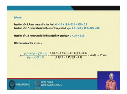
Similarly I have to look at how much of oversize material present into your overflow. So, let us look at the oversize material. So, overflow, in the overflow how much of material which is coarser than 1.5? So, this is a 37 plus 36 is 73 plus 7. So, that is 80 percent or this fraction will be 0.8. So, this is the fraction or plus 1.5 millimetre material in the overflow product that is reported as small p that is equal to 80 percent or equal to 0.8.
