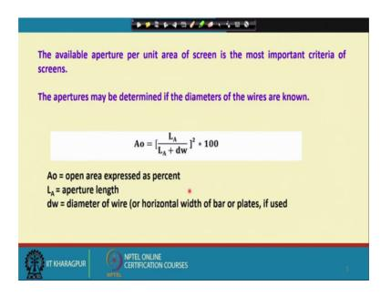
Very important issue for this woven wire screens are the available aperture; that means, what is the available aperture per unit area of screen, is the most important criteria of screens. Because, your screening efficiency will largely depend on how much of the aperture area you have created or you have provided per unit length or per unit area. So, the available aperture per unit area of screen is the most important criteria of screens, but how do we calculate this available aperture area.
