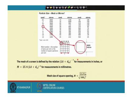
Now, let us see that we are discussing many times about the size with a unit called mesh. Now, these days we try to use it with directly with a micro metres or metres or millimetres like that meters we do not have any screen in that length so, but it is also conventionally being used that is one unit it is called the mesh. Now, what is that mesh? So, mesh is basically of a screen is the defined as what is that your how many numbers of holes are there per unit length.
