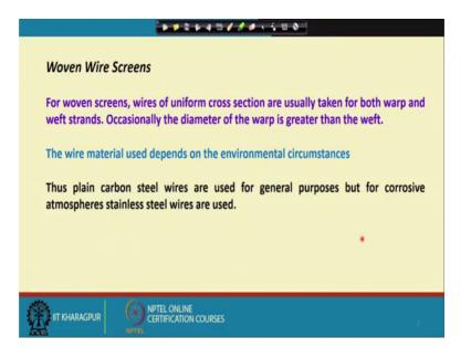
Woven Wire screens will look at the, they are wires of uniform cross section are usually taken for both warp and weft strands; there is a warp, this is the weft. So, basically you have to take uniform cross sections otherwise the aperture sizes will differ and occasionally the diameter of the warp that is what is basically withstanding the maximum load of the particles is greater than the weft.
