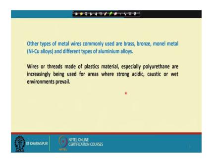
Other types of metal wires commonly used are brass, bronze, monel metal which is a nickel copper alloys at different types of aluminium alloys wires or threads made a plastics material especially polyurethane are increasingly being used for areas where strong acidic caustic or weft environments prevail.
