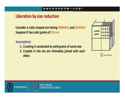
Let us consider a cubic shaped ore having mineral and gangue these are all having a mixture of mineral and gangue and support it has a cubic grains of 10 millimeter each this is a grain sizes I am talking about. Let us assume that we have crossed this material this entire cube to heal grains of same size. Crystals in the ore are intimately joined with each other they are intimately locked that is your mineral and gangue materials. (Refer Slide Time: 23:27)
