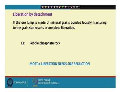
Many times if the old lump is made of mineral grains bonded loosely, fracturing to the grain size results in complete liberation. Like if I have a particle which is basically surrounded by loose, your clay bearing materials. So, if I put some compressive force into that the loose grains will be dislodged and my wanted material will be free from the unwanted material. Example is a pebble phosphate rock and however, mostly liberation needs or requires size reduction.
