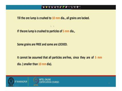
Now, as long as we are crushing and unless we reach to 10 millimeter dia all grains are locked that is the characteristic of that particular deposit which we are discussing as an example. Now, suppose we further cross it to 5 millimeter dia. So, what will happen? Now, some grains may be free and some may be locked, but it cannot be assumed that all particles are free since there of 5 millimeter dia we cannot guarantee that.
