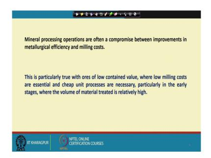
Mineral processing operations are often a compromise between improvements in metallurgical efficiency and milling costs. Why I said compromise scientifically it may be possible to separate them do it in the purest of its form, but what is the efficiency of that that is how much was available in the mind ore and how much you are basically recovering that we will come very soon.
