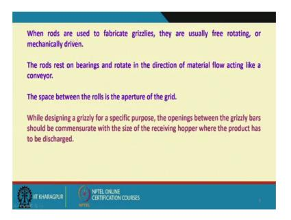
When rods are used that means, it is not always required that you have to use a rail, your steel rails for you are making the grizzlies even you can use the rods, are used to fabricate grizzlies they are usually free rotating type. That means, the rods will
