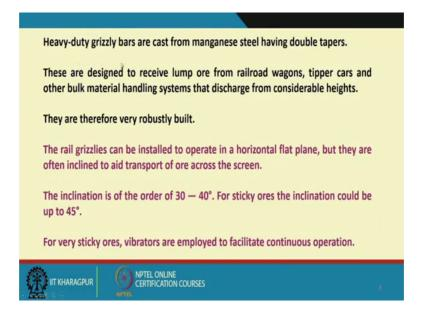
Heavy duty grizzly bars are cast from manganese steel having double tappers that you can have your double tapper also that is you have a taper and then you can have further taper and they are mostly basically made of your cast manganese steel. These are designed to receive lump ore from the railroad wagons tipper cars and other bulk material handling systems that discharge from considerable heights.
