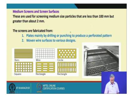
Now, that is about the coarse screens. That is the surfaces and we have structures we have discussed. Now it is called the medium screens; that means, when we are dealing with the medium size fraction; that means, they are not the boulders, they are not directly coming from the mine sites they have already been crossed, they are normally the crossed products.
