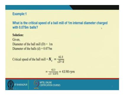
There is an example one the question is what is the critical speed of a ball mill of one meter internal diameter charged with 0.075 meter balls. That means, we are having only one type of ball and that your say diameter of these balls are 0.075 meter and the ball mill diameter is 1 meter. So, we need to calculate what is the critical speed of a ball mill.
