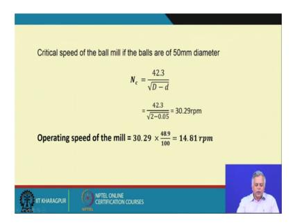
So, critical speed of the ball mill if the balls are of 50 meter millimeter diameter. So, N c that is the critical speed will be equal to 42.3 divided by a square root of capital D minus
