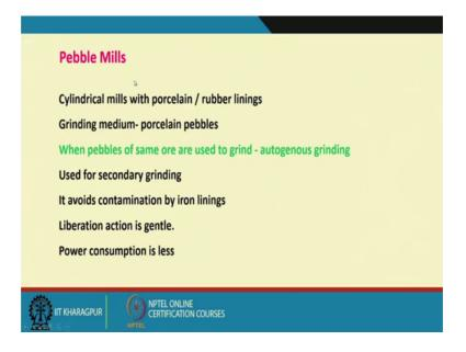
There are also pebble mills, which are basically the cylindrical mills with porcelain or rubber lining. So, we make it because to protect your mill surfaces from the wear.
