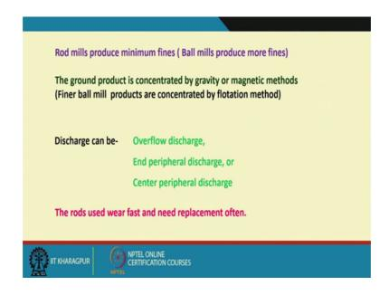
So, rod mills produce minimum fines, why now it tries it tries to break the relatively coarser particles at a faster rate than the finer particles, but in case of ball mills you do not have this type of preferential breakage options because of the mechanism what you are utilizing in a ball mill. So, the ball mill generally generate relatively more proportion of fines than in a rod mill; and in a rod mill product you have got your relatively your closest size range of materials.
