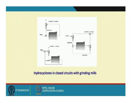
And mostly the as I said the grinding mills are in closed circuit. So, the circuit configuration could be like this. Here we do not use screens because the screens and they
