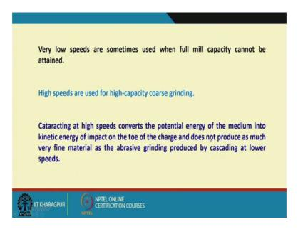
Very low speeds are sometimes used when full mill capacity cannot be attained. Like many a times I have got a mill which can accept up to which can process up to 10,000 tons per hour, but we are not getting input material at that rate we may be getting at 8,000 tons per hour. So, in that case maybe we can reduce the mill speed, so that my capacity is matched.
