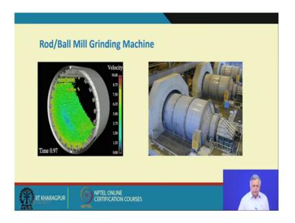
The series this is the animation which is showing how your mill it may be a rod mill, it may be a ball mill how the grinding occurs. So, this is basically your charge material sorry. So, when the charge material is basically rotated and then what will happen everything will falls back will fall back at a different your axis. So, what will happen is because of M b square by R.
