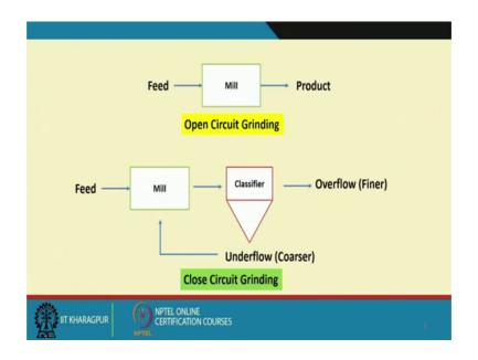
Now, this is the schematic I wanted to show you that what is that open circuit grinding is like a mill. We call it grinding mill. So this is the feed and it is coming there and then it is getting discharged as a product and when it happens like this so that means, we are not controlling any the product quality we call it open circuit grinding.
