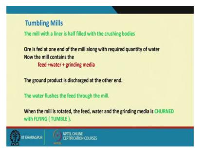
Then where this grinding ah say occurs what are the equipment we use we call them in general that is tumbling mills because they are rotating type of mills. And the mill with a liner because we use a liner that is your grinding surface inside the mill, it is just like you
