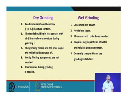
We will discuss it through these comparative statements, like the dry grinding versus wet grinding. The dry grinding is normally your done when the feed material should have low moisture content that is less than one percent.
