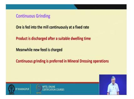
Continuous grinding ore is fed into the mill means is the tumbling mill continuously at a fixed rate so; that means, you have got a mill and it is continuously fed at a particular feed rate and it is getting discharged also at a particular rate.
