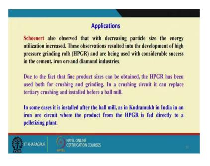
So, professor Sonnet also observed that with the decreasing particle size the energy utilization increased; that means, in relation to other breakage devices. These observations resulted into the development of high pressure grinding roles and are being used with considerable success in the cement iron ore and diamond industries, but HPGR is being researched for much more wider applications for different minerals. There is a
