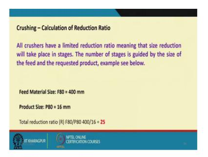
Now, let me discuss now how to calculate the reduction ratio. So, all crushers have a limited reduction ratio what does it mean? That it mean that it means that the size reduction will take place in stages; that means, each crusher is designed to break from a
