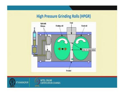
Now, this is another crusher which is relatively new and which is going to revolutionize these combination processes, it has already find it has already been found wide acceptance in many industries this is called a high pressure grinding roll.
