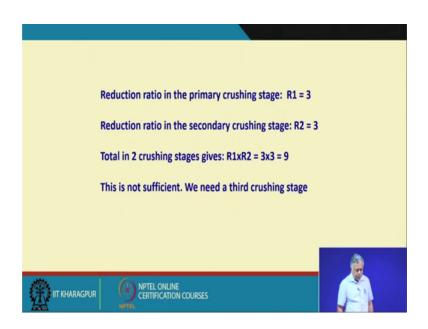
Now, suppose we know the reduction ratio in the primary crushing stage normally, that is around 3 event for the secondary crossing stage in the reduction ratio is three; that means, is F 80 by P 80 is around 3. So, if I have to that is one primary crusher and one secondary crusher. So, my the after secondary after second crushing stages will give me a reduction ratio of R 1 into R 2 that is 3 into 3 that is 9, but our required ratio reduction
