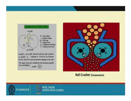
Now if I look at here suppose if I have 2 rolls now and a roll diameter is designated as capital R as suppose the particle we assume that that is a spherical particle and that particle radius is represented as a small r and this angle.
