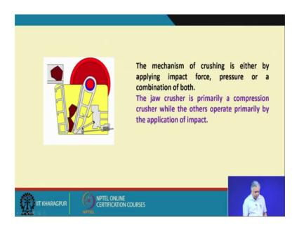
So, this is an animation of how a jaw crusher works; I got it from the open source. So, here you see that this is a fixed jaw and this is a moving jaw and the particles are coming like this. And then they are basically experiencing some kind of your force in between your fixed jaw and the moving jaw. And this opening is called the gate and this discharge; this distance is called the set.
