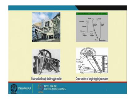
So, if you look at this that this is the call that is seeping area, so this is a basically a jaw crusher and this is the width of this jaw crusher. So, what is the width of that jaw crusher? And to their receive me that the width of the jaw crusher and the gape; that means, what is the basically the distance between the two jaws. So, that is the gape and that is what the width is there; so, you get a cross sectional area of that.
