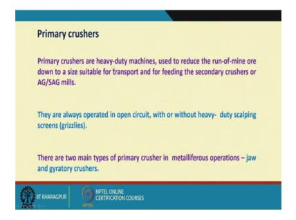
Now, primary crushers they are basically used to reduce the run of mine ore; down to a size, suitable for transport and for feeding the secondary crushers or auto genius grinding or semi auto genus grinding mills; which will discuss in due course of time. So, these are basically used to reduce the run of mine ore; down to a size suitable for transport.
