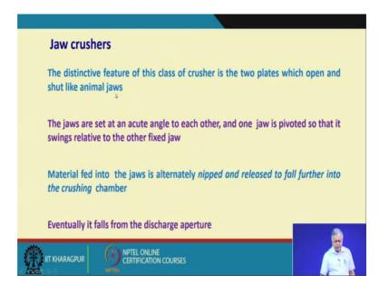
So, jaw crushers is basically the name has come; it has got similarity with the animal jaws. The distinctive feature of this class of crusher is that two plates which open and sort like animal jaws; like even our own jaws; like one jaw is fixed and another jaw is moving and that is how we cross and we have got our teeth to break that particles.
