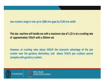
Jaw crushers generally range in size; that means, what are available in the market up to 1680 millimeter gape by 2130 millimeter width. These are what is available as far as I am concerned that is available in the market. This size machine will handle ore with the maximum size of 1.22 meter; that means, the rom ore, which is having a maximum size of 1.22 meter. It can accept that if you have a 1680 millimeter gape and 2130 millimeter
