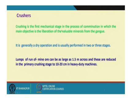
Now first stage is the crusher, we will start with the crushers; so, crushing is a first mechanical stage in the process of comminution, in which the main objective is the liberation of the valuable minerals from the gangue. Actually as I had said already that entire comminution process is primarily focused on liberation of materials where we talk about mineral processing operation. That means, you are preparing your material for subsequent separation.
