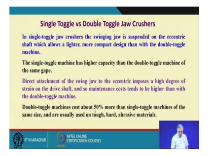
In single toggle jaw crushers, the swinging jaw as I explained is suspended on the eccentric shaft which allows a lighter, more compact design than with the double toggle machine. Because when do we have two rods connecting each other, then you should have a much bigger; your say design or say bigger surface area for the machine to be accommodate it.
