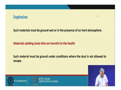
Such materials must be ground wet or in the presence of an inert atmosphere whether the material is explosive in nature. So, in that condition, maybe depending upon the nature of that your root causes for that explosiveness of that material we have to find out. And then depending on the need we may have to process that material either in inert atmosphere or maybe in wet condition.
