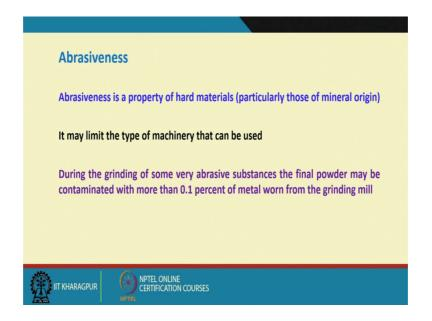
Abrasiveness; abrasiveness is a property of a hard materials, particularly those of mineral. Origin if the material is abrasive. So, it may limit the type of machinery that can be used. Because is the where of the material surface through which I am trying to break that material.
