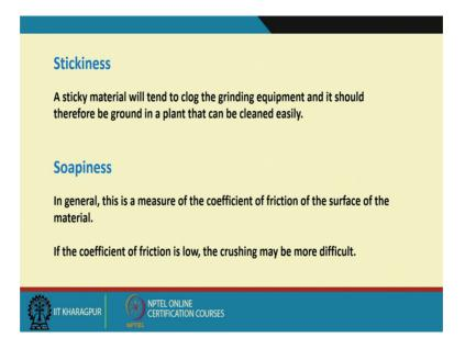
Stickiness we have already discussed, that is sticky material will tend to clog the grinding equipment or say breakage equipment, and it should therefore, be ground in a plant that can be cleaned easily; that means, how do I clean the surface of my equipment through which the basically the force is being applied to break my particles. Otherwise, the applied force may not be transmitted to my particles and the particle breakage will not be satisfactory.
