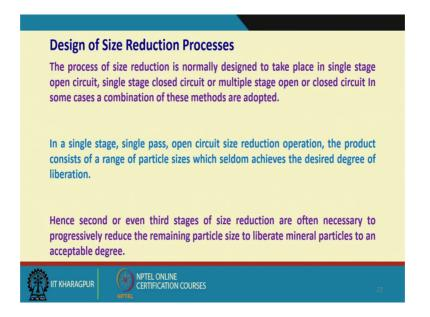
Now coming to this point; that is, how do we design the size reduction process then? The process of size reduction is normally designed to take place in single stage open circuit. Or maybe single stage closed circuit. Or multiple stage open or closed circuit. In some cases a combination of these methods are adopted.
