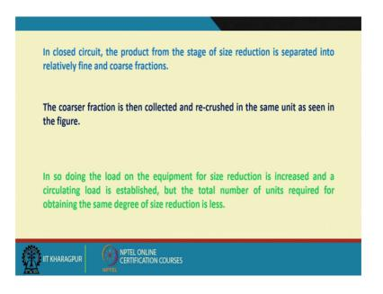
So, in closed circuit, the product from the stage of size reduction is separated into relatively fine and coarse fractions. The coarser fraction is then collected and re crushed in the same unit as seen in the figure I have already discussed it. And while doing so
