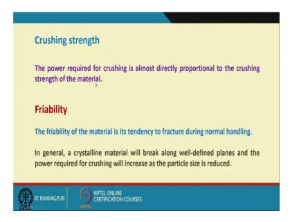
There is another thing called crushing strength. What is the crushing strength? That the power required for crushing is almost directly proportional to the crushing strength of the material.
