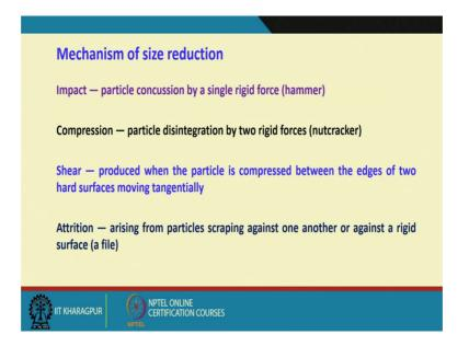
So, if we look at the mechanism of size reduction. And how can you have a size reduction? That means, what are the different machines they are designed based on what mechanism. What is the impact? That is particle concussion by a single digit force like a hammer. So, it is an impact.
