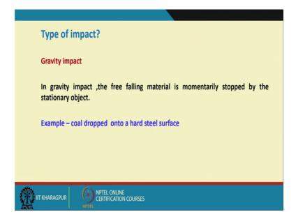
Now, if you will get into this impact, what type of impact? It can be gravity impact. In gravity impact, the pre falling material is momentarily stopped by the stationary object. Like a material is flowing like this, and it is stopped momentarily, and then you are putting a putting an impact into that.
