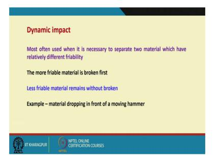
will show you some equipment into course of time. When do we need compression forces? Now if the material is very hard. If the material is abrasive, if the material is not sticky, because what will happen if the material is sticky because we are trying to compressed it. So, if the material is sticky. So, what will happen? Some portion of this material will get added to the surface of that you are breaking up that material through which you are trying to break the particles; so the relative.
