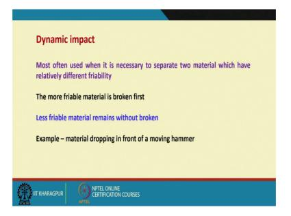
Then we can have dynamic impact. Most often used when it is necessary to separate 2 material, which have a relatively different friability. Like I know that I have got a heterogeneous particle assemblage, but one material is friable another one is hard material is not friable. So, there we can have a dynamic impact. Because what will happen the more friable material will be broken for us, so that means, we are having a preferential breakage.
