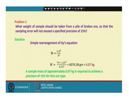
So, that is why I have given this problem that what weight of samples should be taken from a pile of broken ore.
