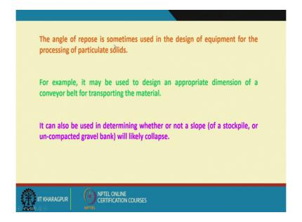
We were talking about the application of angle of repose. Angle of repose sometimes used in the design of equipment for the processing of particulate solids that is if I am using a as I said that your say conveyor belt that is we can appropriately design or say decide about the dimension of a conveyor belt if we know the angle of repose of that material.
