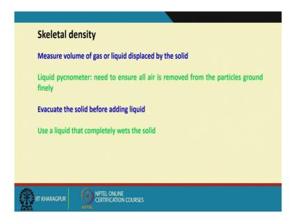
Now one type that is called skeletal density, skeletal density is the basically what I said here that is the density of true density, so skeletal density how do I know again the same principle I will be using that is displacement of fluid basis and what is the volume of that fluid I have displaced. But imagine that you are given a particle whose size is 10 micrometer, now if I try to displace water can we really measure the volume of that water how much it is displaced almost impossible.
